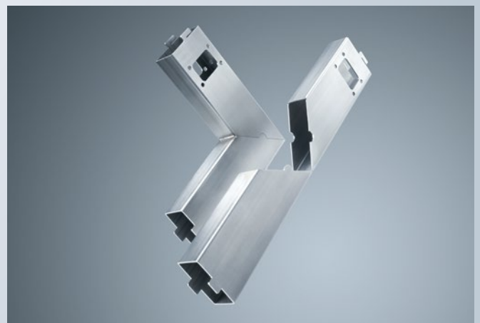
Efficient production of bend connections and positioning aids using a laser.
