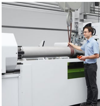
Ideal for lot sizes of 1: Crane loading also possible for heavier tubes.
