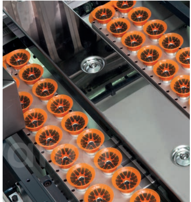
Suction plates in gauge table with 4 suction units (from 3200 mm with 6 suction units), controlled via the software POS 3000.
