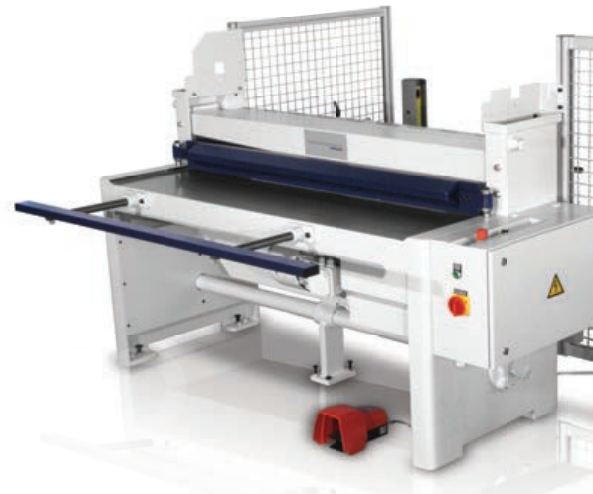
Standard: MSHU with rear guarding via 2-beam light barrier incl. side protection grid
