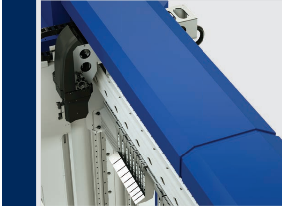
Two rotating units with one gripper arm each remove the tools from the magazine
