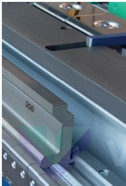
Bottom beam blade with finger tools
