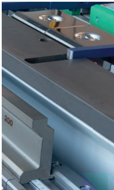
Bottom beam blade with finger grooves
