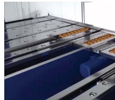
U-gauge with balls in table and suction gauge for smooth handling of the sheet
