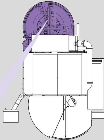
**Mikron MILL S 600 U: disc-type magazine**
