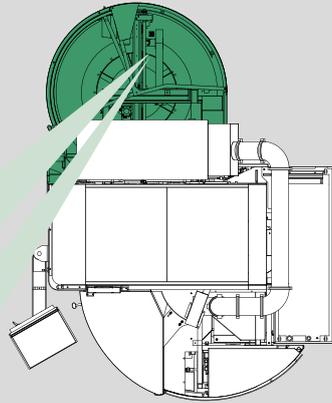
**Mikron MILL S 400 / 400 U: disc-type magazine**
