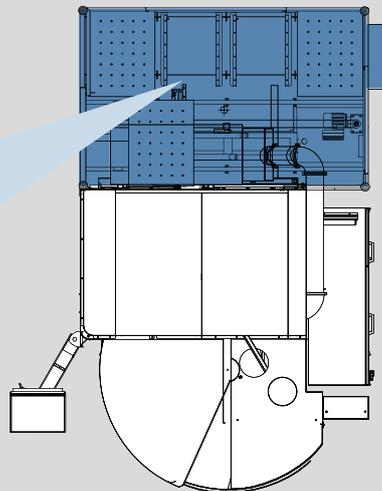
**Mikron MILL S 600 / 800: linear-type magazine**
