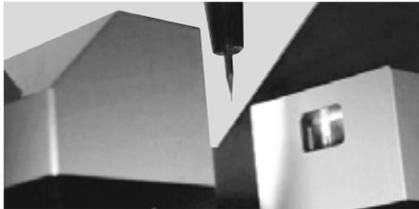
True tool measurement thanks to digital cleaning of foreign objects (particles and chips).
