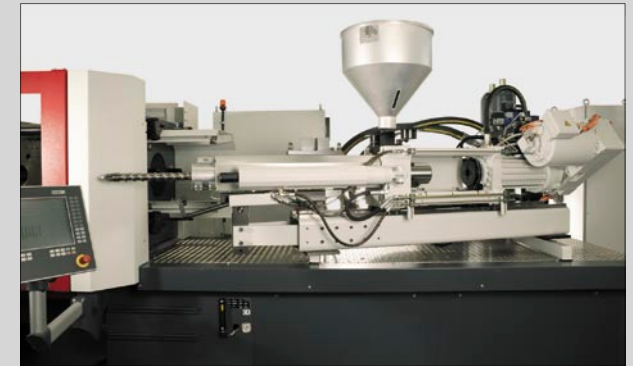
Injection unit swivels for easy maintenance
