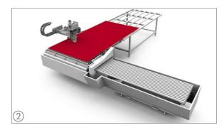
The table is fed into the cutting area automatically. The parts in the first segment are cut.
