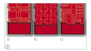
With the ByVention, the sheet is divided up into segments that are processed one after another. This accounts for the **three** different strategies that can be used to nest parts on the sheet.
