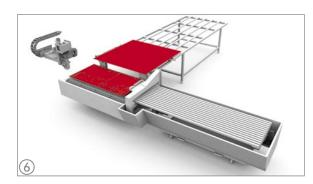
The finished table segment is placed on the removal table automatically. This procedure repeats until the entire sheet has been processed. As soon as the last segment of the table is in the cutting area, a new sheet can be placed on the loading table.
