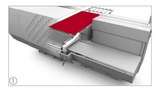
The metal sheet is placed on the loading table manually and pushed up to the table stop.
