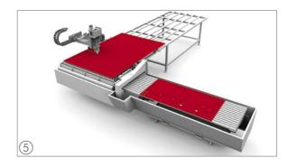
The removal table carries the finished table segment automatically from the cutting area to the removal area. At the same time, the sheet is fed into the cutting area so that the next segment can be cut. The cut parts as well as the partly cut sheet are now taken manually from the removal area.
