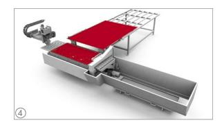
The finished table segment is placed on the removal table automatically.
